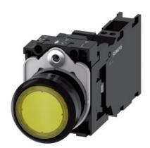
Illuminated pushbutton, 22 mm, round, plastic, yellow, pushbutton, flat, momentary contact type, with holder, 1 NO+1 NC, LED module with integrated LED 110 V AC, spring-type terminal, with laser labeling, symbol number according to, ISO 7000 or IEC 60417
