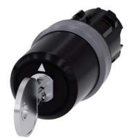
key-operated switch Siemens, 22 mm, round, plastic with metal front ring, special lock, with 2 keys, 3 switch positions I-O<II, left latching, momentary contact type on the right, actuating angle  $2x45^{\circ}$ , 10:30h/12h/13:30h, key removal O
