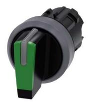
Selector switch, illuminable, 22 mm, round, plastic with metal front ring, green, selector switch, short, 3 switch positions I-O<II, left latching, right momentary contact type, actuating angle 2x45°, 10:30h/12h/13:30h, with laser labeling, upper case and lower case, always upper case at the beginning of the word
