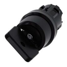
Key-operated switch O.M.R, 22 mm, round, plastic, lock number 73034, black, with 2 keys, 2 switch positions O-I, latching, actuating angle  $90^\circ, 10:30h/13:30h$ , key removal O+I, with laser labeling, inscription or symbol Customer-specific selection with SIRIUS ACT configurator (CIN)
