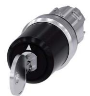
key-operated switch Siemens, 22 mm, round, metal, shiny, lock number SSG10, with 2 keys, 3 switch positions I-O-II, latching, actuating angle 2x45°, 10:30h/12h/13:30h, key removal I+O+II, with laser labeling, upper case
