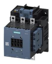
Traction contactor, AC-3 185 A, 90 kW / 400 V Coil 24 V DC x (0.7-1.25) PLC input 24-110 V DC Auxiliary contacts 2 NO + 2 NC 3-pole size S6 Busbar connections Coil connection: Spring-type terminal
