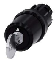
Key-operated switch BKS, 22 mm, round, plastic, lock number S1, with 2 keys, 3 switch positions I-O-II, latching, actuating angle 2x45°, 10:30h/12h/13:30h, Key removal I+O+II, with laser labeling, upper case and lower case, always upper case at the beginning of the word
