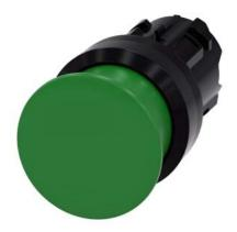
Mushroom pushbutton, 22 mm, round, plastic, green, 30 mm, momentary contact type, with laser labeling, upper case and lower case, always upper case at the beginning of the word
