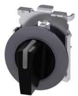
Illuminable selector switch, 30 mm, round, Metal matt, black, Selector switch short, front ring for flush installation, latching, actuating angle 2x45°, 10:30 /12 /13:30, Z=50-unit packaging
