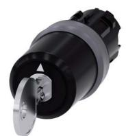
key-operated switch Siemens, 22 mm, round, plastic with metal front ring, special lock, with 2 keys, 3 switch positions I-O-II, latching, actuating angle 2x45°, 10:30h/12h/13:30h, key removal II
