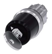
key-operated switch Siemens, 22 mm, round, metal, shiny, lock no. LSG1, with 2 keys, 2 switch positions O<I, momentary contact type, actuating angle 45°, 10:30h/12h, key removal O, with laser labeling, upper case and lower case, always upper case at beginning of line
