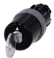
key-operated switch Siemens, 22 mm, round, plastic with metal front ring, lock number SSG10, with 2 keys, 3 switch positions I-O-II, latching, actuating angle 2x45°, 10:30h/12h/13:30h, key removal O+I, with laser labeling, lower case
