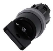
Key-operated switch O.M.R, 22 mm, round, plastic with metal front ring, lock number 73034, black, with 2 keys, 2 switch positions O-I, latching, actuating angle 90°, 10:30h/13:30h, key removal I, with laser labeling, upper case
