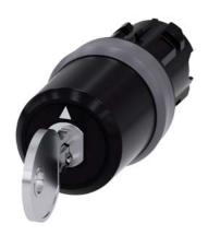
key-operated switch Siemens, 22 mm, round, plastic with metal front ring, lock number SSG10, with 2 keys, 3 switch positions I-O-II, latching, actuating angle  $2x45^{\circ}$ , 10:30h/12h/13:30h, key removal I, with laser labeling, upper case and lower case, always upper case at the beginning of the word
