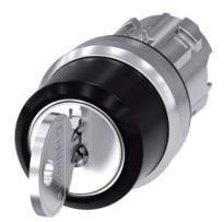
RONIS key-operated switch, 22 mm, round, metal, shiny, lock number SB30, with 2 keys, 3 switch positions I-O<II, left latching, right momentary contact type, actuating angle 2x45°, 10:30h/12h/13:30h, key removal O, possible special locks: SB31, 421, 455, Z=50-unit packaging
