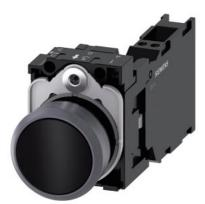
Pushbutton, 22 mm, round, plastic with metal front ring, black, pushbutton, flat, momentary contact type, with holder, 1 NO+1 NC, spring-type terminal, with laser labeling, upper case
