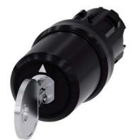
key-operated switch Siemens, 22 mm, round, plastic, lock number SSG10, with 2 keys, 3 switch positions I>O<II, momentary contact on the left, latching on the right, actuating angle 2x45°, 10:30h/12h/13:30h, key removal O+II, with laser labeling, upper case and lower case, always upper case at beginning of line
