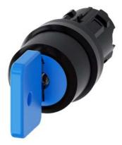
Key-operated switch O.M.R, 22 mm, round, plastic, lock number 73038, blue, with 2 keys, 3 switch positions I-O-II, latching, actuating angle 2x45°, 10:30h/12h/13:30h, Key removal I+O+II Z=50-unit packaging
