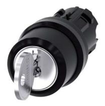
RONIS key-operated switch, 22 mm, round, plastic, lock number SB30, with 2 keys, 3 switch positions I>O<II, momentary contact on the left, latching on the right, actuating angle 2x45°, 10:30h/12h/13:30h, Key removal O+II, possible special locks: SB31, 421, 455, with laser labeling, upper case
