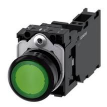
Illuminated pushbutton, 22 mm, round, plastic, green, pushbutton, flat, momentary contact type, with holder, 1 NO+1 NC, LED module with integrated LED 110 V AC, spring-type terminal, Z=20-unit packaging
