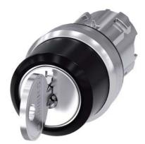
RONIS key-operated switch, 22 mm, round, metal, shiny, lock number SB30, with 2 keys, 3 switch positions I-O-II, latching, actuating angle 2x45°, 10:30h/12h/13:30h, Key removal II, possible special locks: SB31, 421, 455, with laser labeling, upper case and lower case, always upper case at the beginning of the word
