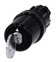
key-operated switch Siemens, 22 mm, round, plastic, lock number SSG10, with 2 keys, 3 switch positions I-O<II, left latching, momentary contact type on the right, actuating angle  $2x45^{\circ}$ , 10:30h/12h/13:30h, key removal O+I, with laser labeling, upper case
