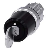
Key-operated switch BKS, 22 mm, round, metal, shiny, lock number S1, with 2 keys, 3 switch positions I-O<II, left latching, right momentary contact type, actuating angle  $2x45^{\circ}$ , 10:30h/12h/13:30h, key removal O+I, with laser labeling, upper case
