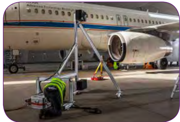
Fig. 4: Installation of DLR's mobile large-scale PIV facility system for flow velocity measurements in the vicinity of the DLR-ALTA research aircraft.
