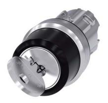
RONIS key-operated switch, 22 mm, round, metal, shiny, lock number SB30, with 2 keys, 2 switch positions O<I, momentary contact type, Actuating angle 45°, 10:30h/12h, key removal O, possible special locks: SB31, 421, 455, with laser labeling, upper case and lower case, always upper case at beginning of line
