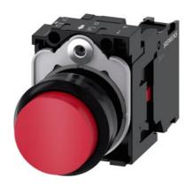
Pushbutton, 22 mm, round, plastic, red, pushbutton, raised, momentary contact type, with holder 1 NC, screw terminal, Z=20-unit packaging
