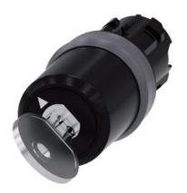
Key-operated switch BKS, 22 mm, round, plastic with metal front ring, lock number S1, with 2 keys, 2 switch positions O-I, latching, actuating angle 90°, 10:30h/13:30h, key removal O+I, with laser labeling, upper case and lower case, always upper case at beginning of line
