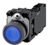
Illuminated pushbutton, 22 mm, round, plastic with metal front ring, blue, pushbutton, flat, momentary contact type, with holder, 1 NO+1 NC, LED module with integrated LED 24 V AC/DC, screw terminal, with laser labeling, inscription or symbol Customer-specific selection with SIRIUS ACT configurator (CIN)
