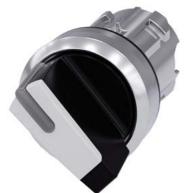
Selector switch, illuminable, 22 mm, round, metal, shiny, white, selector switch, short, 2 switch positions O-I, latching, actuating angle 90°, 10:30h/13:30h, Z=50-unit packaging
