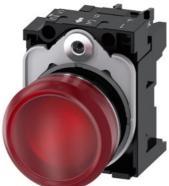
Indicator lights, 22 mm, round, Metal, shiny, red, lens, smooth, with holder, LED module with integrated LED 230 V AC, screw terminal, with laser labeling, inscription or symbol Customer-specific selection with SIRIUS ACT configurator (CIN)
