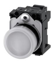
Indicator light, 22 mm, round, plastic, white, lens, smooth, with holder, LED module, with integrated LED 230 V AC, spring-type terminal, with laser labeling, upper case and lower case, always upper case at beginning of line
