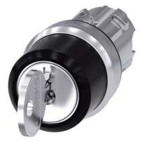
RONIS key-operated switch, 22 mm, round, metal, shiny, lock number SB30, with 2 keys, 3 switch positions I-O-II, latching, actuating angle 2x45°, 10:30h/12h/13:30h, Key removal I+O+II, possible special locks: SB31, 421, 455, with laser labeling, upper case and lower case, always upper case at the beginning of the word
