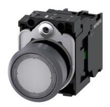
Illuminated pushbutton, 22 mm, round, plastic with metal front ring, clear, pushbutton, flat, momentary contact type, with holder, 1NO, LED module with integrated LED 110 V AC, screw terminal, with laser labeling, symbol number according to, ISO 7000 or IEC 60417
