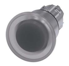
Illuminated mushroom pushbutton, 22 mm, round, metal, shiny, clear, 40 mm, latching, pull-to-unlatch mechanism, with laser labeling, symbol number according to, ISO 7000 or IEC 60417
