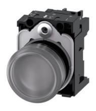
Indicator lights, 22 mm, round, plastic, clear, lens, smooth, with holder, LED module, with integrated LED 230 V AC, screw terminal, with laser labeling, upper case and lower case, always upper case at the beginning of the word
