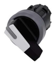
Selector switch, illuminable, 22 mm, round, plastic with metal front ring, white, selector switch, long, 2 switch positions O-I, latching, actuating angle 90°, 10:30h/13:30h, with laser labeling, upper case and lower case, always upper case at the beginning of the word
