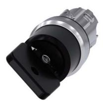
Key-operated switch O.M.R, 22 mm, round, metal, shiny, lock number 73034, black, with 2 keys, 2 switch positions O-I, latching, actuating angle 90°, 10:30h/13:30h, key removal I, with laser labeling, inscription or symbol Customer-specific selection with SIRIUS ACT configurator (CIN)
