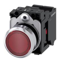
Illuminated pushbutton, 22 mm, round, Metal, shiny, red, pushbutton, flat, momentary contact type, with holder, 1 NC, LED module with integrated LED 230 V AC, spring-type terminal, with laser labeling, inscription or symbol Customer-specific selection with SIRIUS ACT configurator (CIN)
