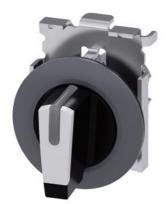
Selector switch, illuminable, 30 mm, round, Metal, matte, white, selector switch, short, front ring for flush installation, 3 switch positions I-O-II, latching, actuating angle 2x45°, 10:30h/12h/13:30h, Z=50-unit packaging
