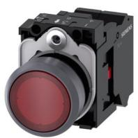
Illuminated pushbutton, 22 mm, round, plastic with metal front ring, red, pushbutton, flat, momentary contact type, with holder, 1NC, LED module with integrated LED 24 V AC/DC, spring-type terminal, with laser labeling, upper case and lower case, always upper case at beginning of line
