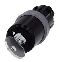
key-operated switch Siemens, 22 mm, round, plastic with metal front ring, lock no. LSG1, with 2 keys, 2 switch positions O<I, momentary contact type, actuating angle 45°, 10:30h/12h, key removal O, with laser labeling, inscription or symbol customer-specific selection with SIRIUS ACT configurator (CIN)
