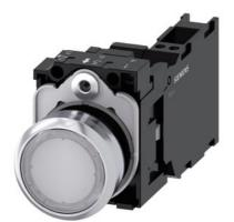
Illuminated pushbutton, 22 mm, round, Metal, shiny, white, pushbutton, flat, momentary contact type, with holder, 1 NO+1 NC, LED module with integrated LED 230 V AC, spring-type terminal, with laser labeling, upper case
