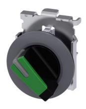
Selector switch, illuminable, 30 mm, round, Metal, matte, green, selector switch, short, front ring for flush installation, 2 switch positions O<I, momentary contact type, Actuating angle 45°, 10:30h/12h, with laser labeling, lower case
