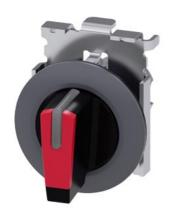
Selector switch, illuminable, 30 mm, round, Metal, matte, red, selector switch, short, front ring for flush installation, 3 switch positions I-O-II, latching, actuating angle 2x45°, 10:30h/12h/13:30h, with laser labeling, lower case
