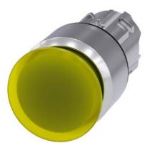
Illuminated mushroom pushbutton, 22 mm, round, metal, shiny, yellow, 30 mm, latching, pull-to-unlatch mechanism, with laser labeling, upper case and lower case, always upper case at the beginning of the word
