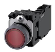
Illuminated pushbutton, 22 mm, round, plastic with metal front ring, red, pushbutton, flat, momentary contact type, with holder, 1 NO+1 NC, LED module with integrated LED 24 V AC/DC, screw terminal, with laser labeling, inscription or symbol Customer-specific selection with SIRIUS ACT configurator (CIN)
