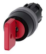
Key-operated switch O.M.R, 22 mm, round, plastic with metal front ring, lock number 73037, red, with 2 keys, 3 switch positions I-O-II, latching, actuating angle 2x45°, 10:30h/12h/13:30h, key removal O+I, with laser labeling, upper case and lower case, always upper case at beginning of line
