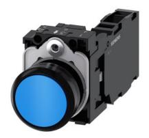
Pushbutton, 22 mm, round, plastic, blue, pushbutton, flat, momentary contact type, with holder 1 NO+1 NC, screw terminal, with laser labeling, lower case
