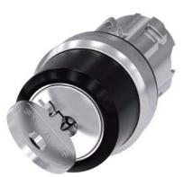
RONIS key-operated switch, 22 mm, round, metal, shiny, Lock No. 421, with 2 keys, 2 switch positions O-I, latching, actuating angle 90°, 10:30h/13:30h, key removal O+I, with laser labeling, inscription or symbol Customer-specific selection with SIRIUS ACT configurator (CIN)
