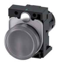
Indicator light with LED lamp, compact, 22 mm, round, plastic, clear with red-yellow-green LED, lens, smooth, with holder, operating voltage 6-24 V AC/DC, screw terminal, with laser labeling, upper case and lower case, always upper case at beginning of line
